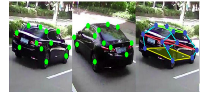
Car orientation detection Use the orientation to dynamically guide user to capture car 360 degree video
